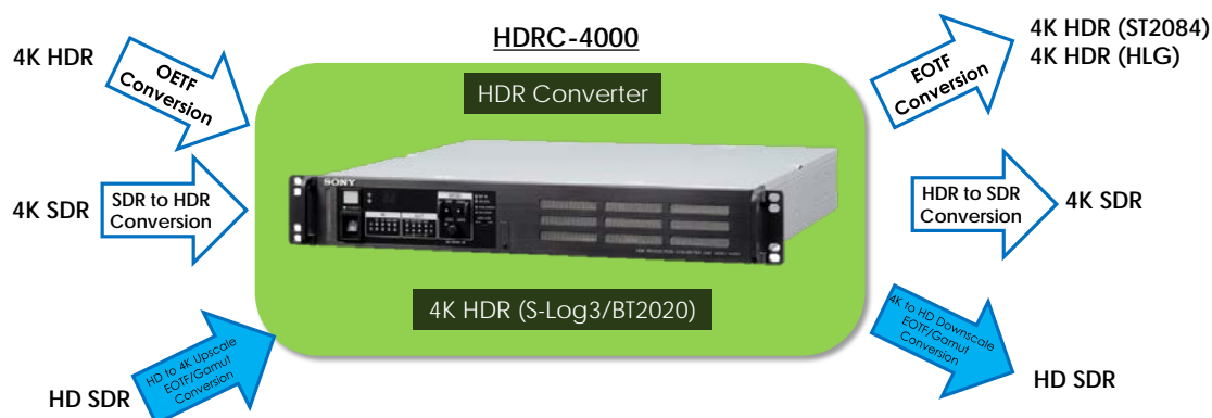
Figure 6: Precision Conversion to/from 4K S-Log3 HDR
