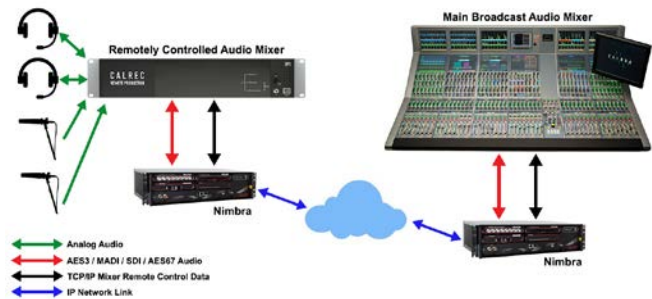
FIGURE 7: AUDIO AND REMOTE CONTROL FOR AT-HOME PRODUCTION
