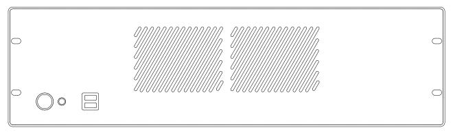
Unit dimensions: 482mm (19") W x 133mm (3U) H x 300mm D Unit weight: 5,5 kg
