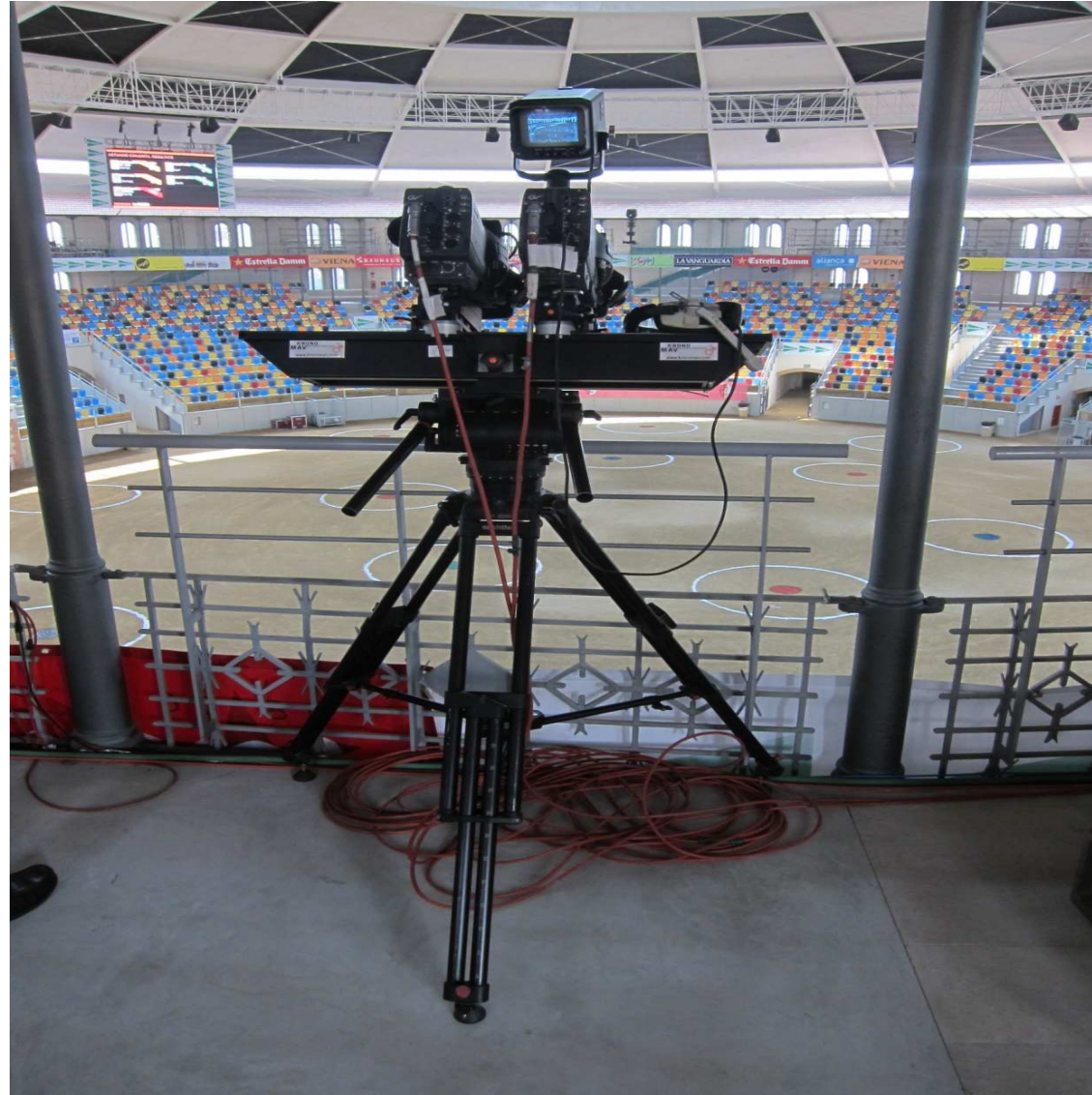
FIXED RIG WITH WIDER RANGE OF INTEROCULAR
