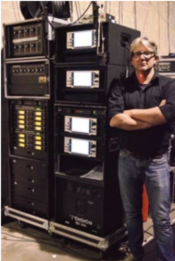
FOH engineer Guido Olischlager played a vital role in the design of the audio system. He is pictured beside the rack of Digital 9000 receivers, 2000 IEM transmitters and Sennheiser Benelux' custom-built antenna combiners
