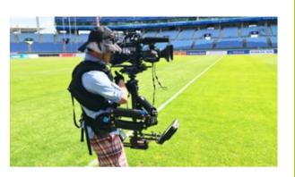
with Gearhouse Broadcast engineers developing a unique solution for the Hitachi SK-HD1200 camera systems. Previously not used over RF, the firmware of the cameras control units was upgraded and GearhouseActis built specially designed brackets to fit wireless transmitters onto the cameras.
