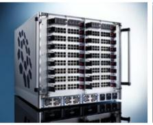
BSkvB runs four modular ControlCenter-Digital matrix switches with 288 ports each.
